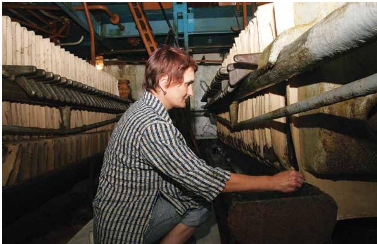
▲ Changing a filter made from sail cloth on a production line at the Svatorskoe Maslo sunflower oil factory in Svatovo, Ukraine. Ukraine is the world's leading sunflower oil producer and exporter. ©Northfoto/Shutterstock
