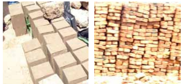
Curing SSB and burnt bricks
