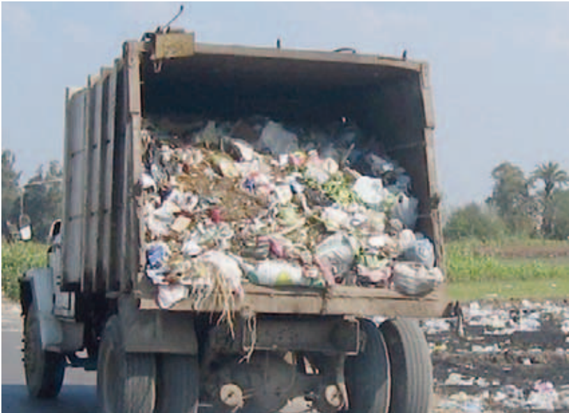
This vehicle used to be a compactor truck. When the compaction mechanism failed the rest of the truck was still operational, so the compacting mechanism was removed.
