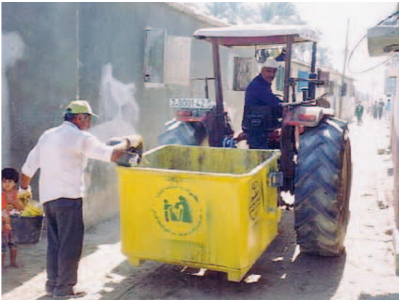
Tractor trailed bins can simplify problems of door to door waste collection.
