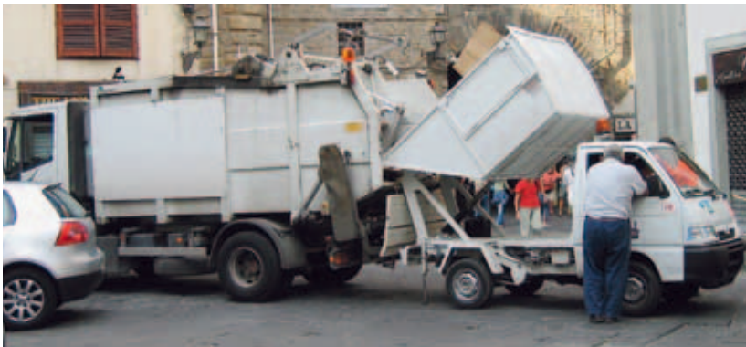
These small trucks sometimes unload directly into a larger truck which takes the waste to the disposal site.
