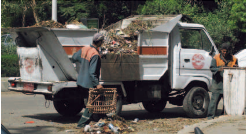
Small tipper trucks are easy to load. In some situations they are very suitable for primary collection.
