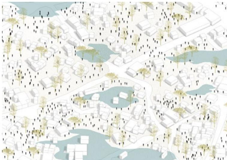
At this stage, flooding is caused due to the natural drainage limitations and topography characterized by a flat and low-lying terrain. The absence of natural slopes and adequate drainage channels exacerbates the retention of surface water following heavy rains.
