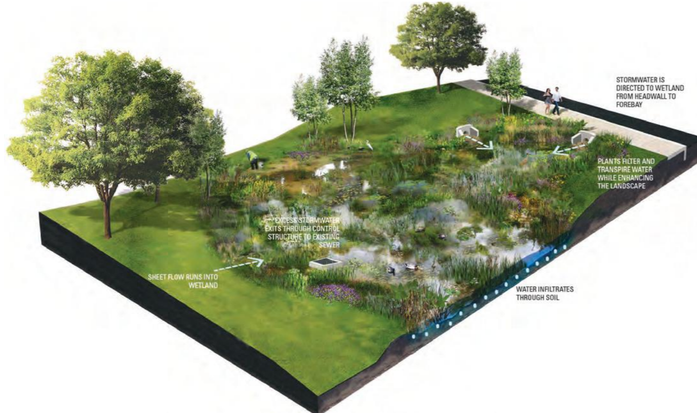
Figure 17. Example of a bio-swale for stormwater collection Source: water.phila.gov/gsi/tools/wetland/
