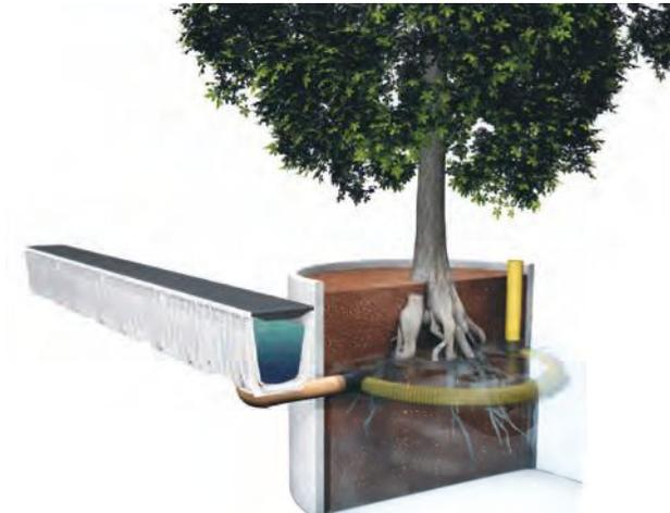
Figure 96. Example of subsurface irrigation system
