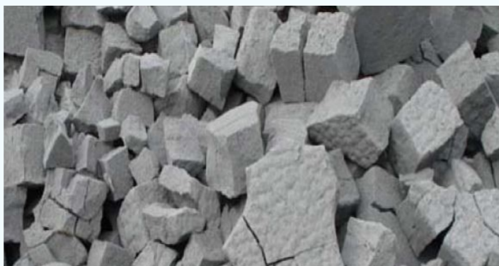
FIGURE 3-7 Glass foam as an option to use glass as a secondary material
