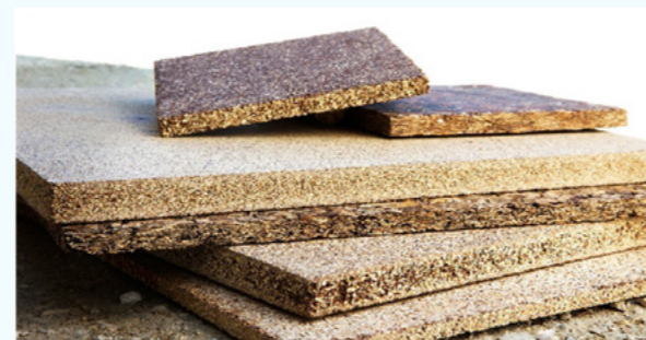
FIGURE 3-22 Composite panel produced with organic waste 59
