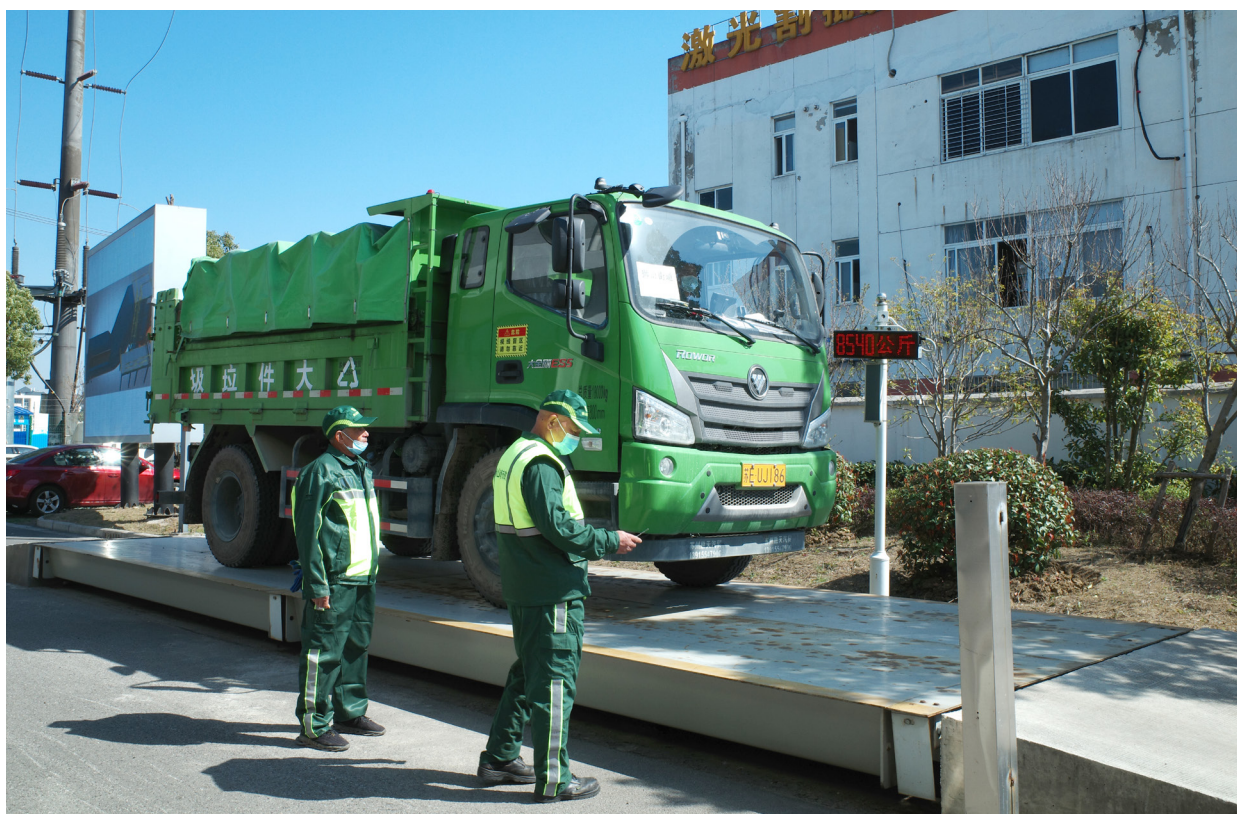
Figure 2-12 Weighing of bulky waste collection vehicle entering the disposal station © UN-Habitat | BAO Meng
