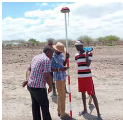
Top right: Beaconing process of Kalobeyei Settlement to mark the boundary of the site. © UN-Habitat
