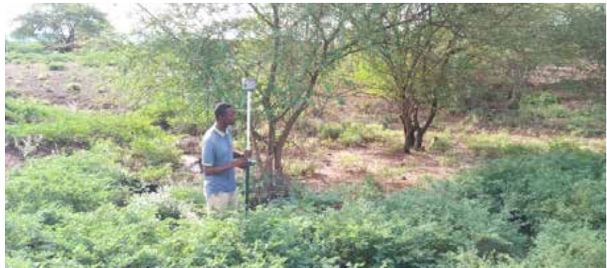
Top right: Surveyor Staking out Spot Heights. © UN-Habitat
