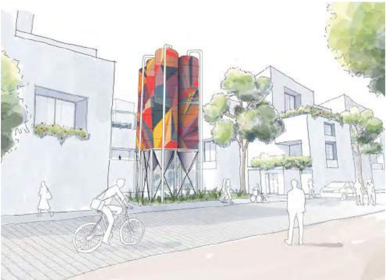
Fig 55. Repurposing of the existing structures to be used as water storage tanks for the irrigation of green spaces/community gardens
