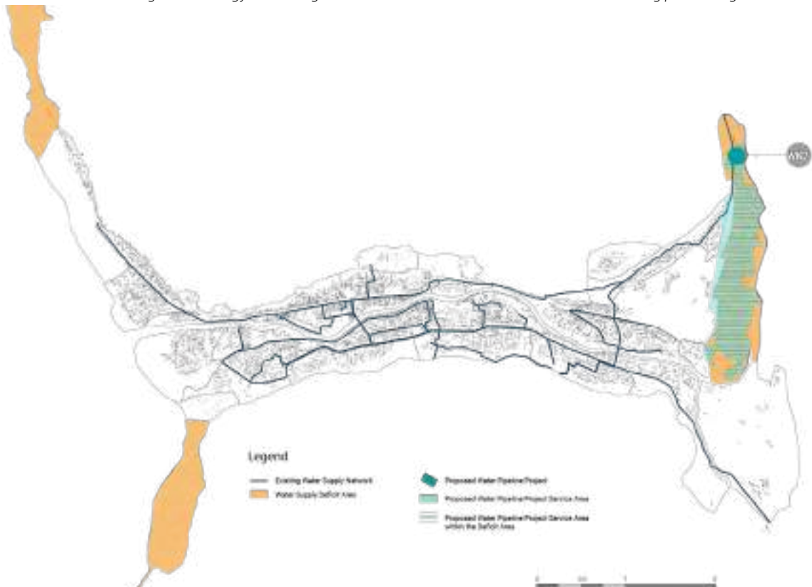
Fig 20. Water Supply Deficit Area Map & Proposed Water Project Service Area. This water supply map represents an example of the deficit assessment and scoring methodology – all categories within Utilities follow the same scoring process against this criteria.
