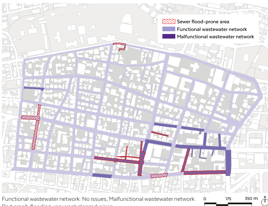
Figure 40 Street mapping of wastewater network
